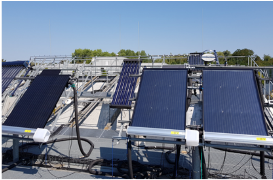
Figure 3.10: Outdoor testbench with the investigated PVT collectors [Jonas et al., 2019].
